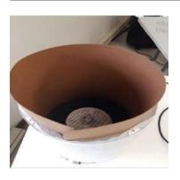
3. IN ORDER TO INSTALL THE CARBON FILTER, YOU NEED TO USE A CARDBOARD THE PROVIDED SLIDER. PUT THE SLIDER INSIDE THE FILTER COMPARTMENT AND GENTLY SPREAD IT AGAINST THE PREFILTER
