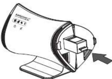
2. When the cartridge is properly installed, you get the beep, and the red cartridge alarm indicator is turned off. The product stays in off mode.
