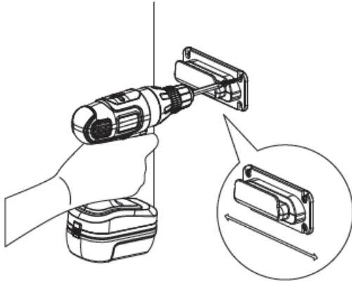
2. Remove the stand base and connect to the wall mount bracket.
