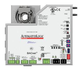
The ZN341V+ is a fully programmable, native BACnet Advanced Application Controller that provides zone level temperature and air quality control for pressure-independent VAV applications. Sophisticated preengineered control algorithms reduce energy consumption, extend actuator life, and increase occupant comfort. It communicates on an EIA-485 LAN using BACnet MS/TP or BACnet over ARCNET communications and connects seamlessly to the WebCTRL® building automation system.
