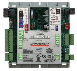
The ZN253 is a fully programmable, native BACnet Advanced Application Controller (AAC) designed for controlling a single zone in a building. The ZN253 is well suited for unit ventilator and packaged HVAC applications that require multiple analog outputs for modulating valves or dampers. It communicates on an EIA-485 LAN using BACnet MS/TP or BACnet over ARCNET communications and connects seamlessly to the WebCTRL® building automation system.
