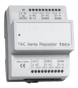
The TAC Xenta® Repeater FTT-10 is a physical layer repeater unit which amplifies the signal on a LonWorks® FT-10 network cable, but does not affect the traffic in any other way.
