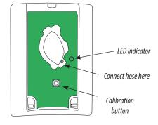
4. Continue flowing gas through the sensor until the LED is off. Estimated calibration time is 5 minutes. Remove hose from calibration port when complete.
