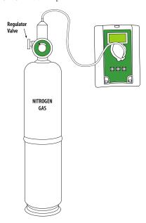
3. Calibrate for 5 min. Unit will return to working display when finished.
