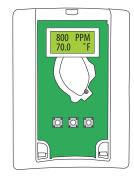
4. When unit returns to working display, remove hose from calibration port and enter Calibration mode as described in the Installation section.
