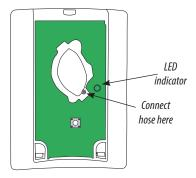
2. Start flowing nitrogen gas (0 ppm CO<sub>2</sub>). Use a flow rate of 0.3 to 0.5 liter/minute.
