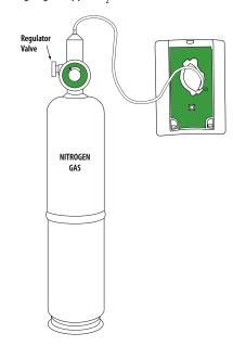
3. Push and hold down calibration button until the LED illuminates.
