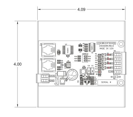
24 VAC to the binary inputs. Higher voltages will damage the expansion module and possibly other components on the system.
