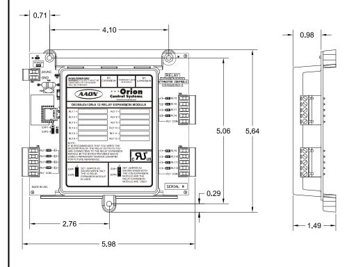
ration jumper is located on the edge of the 12 Relay Expansion Module on the same side of the module as the power connection.
