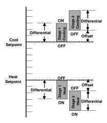
is the difference between the on and off points. This value depends on the load and on the equipment size. If the equipment is large for the load, you may want to make this value as high as 5 to prevent equipment cycling. If the equipment is small compared to the load, or if tight control is desired, you may want to make this value as low as 1.
