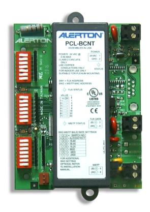
The IBEX/BACnet protocol converter link (PCL-BCNT) enables IBEX systems to communicate with BACnet-compliant devices. The PCL-BCNT is installed between an IBEX TUX trunk and a BACnet MS/TP network, translating object and property data from a single BACnet device to IBEX TUX points.
