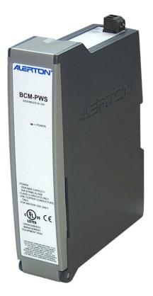
The Alerton<sup>®</sup> BCM-PWS is the base device for Alerton BACtalk control modules (BCMs), providing power for up to seven BCMs. The BCM-PWS requires a 24 VAC power supply. It then conditions power and provides battery backup through a simple ribbon-cable connection to BCMs.
