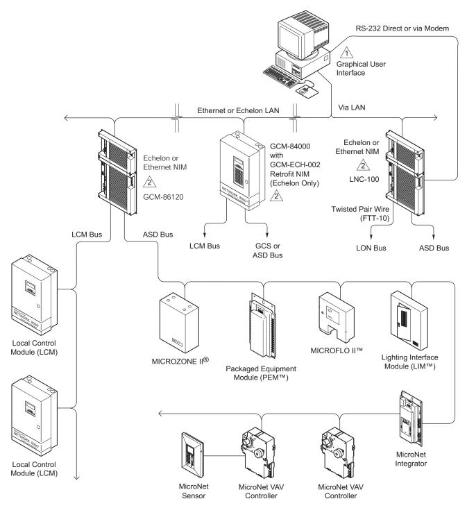
1 Invensys graphical user interfaces use various methods to communicate with the GCM series and LNC controllers. Refer to information in this diagram that is applicable to the chosen user interface.
