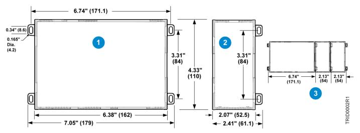
Compatible with (DIN43880) enclosures. Suitable for mounting to a panel or to an EN50022 standard 35 mm rail.
