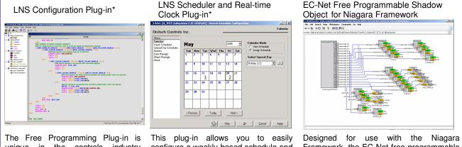
unique in the controls industry because it combines the easy to use graphical interface with the power and flexibility of a code editor and compiler. Distech Controls' Free Programming Plug-In uses a unique and simplified version of BASIC that we have developed in-house and that is custom made to suit control requirements.
