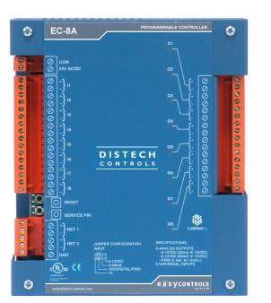
The EasyControls<sup>™</sup> EC-8 controller is a microprocessor based free programmable controller designed to control various HVAC applications. Moreover, it is suitable for any lighting control and power measurement application.
