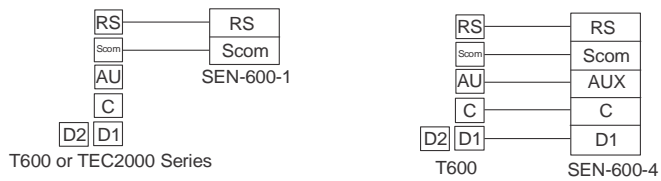
This is a wiring example of a single remote room sensor (S1=On, S2=On).
