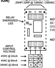
NOTE: INPUT POWER SUPPLY SHOULD BE UL LISTED FOR FIRE PROTECTION SIGNALING SYSTEMS WHEN USED IN FIRE ALARM APPLICATIONS
