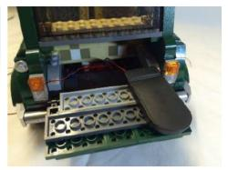
Let the **Coin Cell Battery Pack** rest in the boot. Close the boot and rest the car on its side so you can access the bottom of the car.
