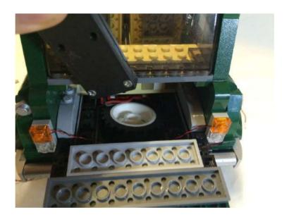
Still holding the **Coin Cell Battery Pack** up and out of the way, refit the floor section of the boot.
