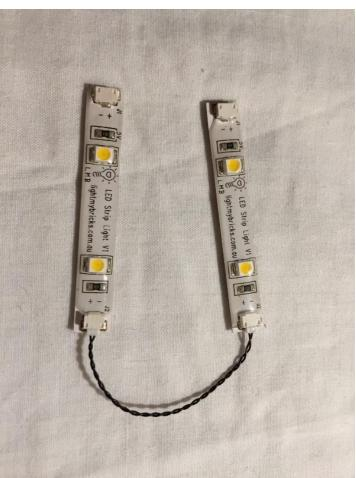
Connect the two **Strip Lights** using the **5cm Connecting Cable**.
