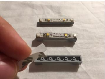
Peel the adhesive backing off the **Strip Lights** and stick them to the back of each of the **Lego Light Grey 1**  $\times$  **6 Plates**.
