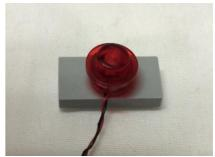
Grab one of the **White Bit Lights** and rest it over the stud on the  $1 \times 2$  modified plate. Position it so that the wire comes down from the middle similar to that in the picture above. Gently place the **Lego Trans Red 1**  $\times$  **1 Round Plate** over the **White Bit Light**.
