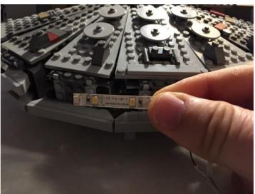
Peel the backing off the **Strip Lights** and in the middle of the joins of each section that had the  $1 \times 6$  tiles (and joined bricks) prepare to stick the **Strip Lights** on.
