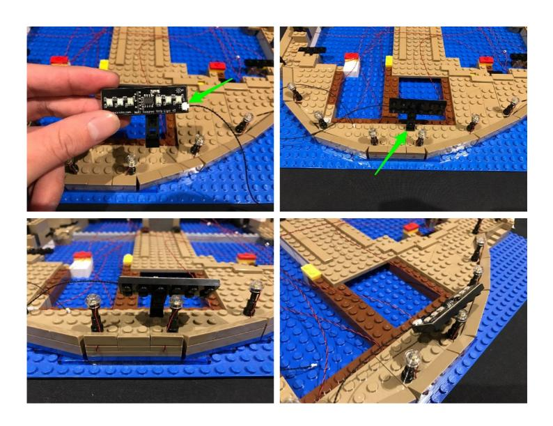
15.) Take the connecting cable from the strip light and then loop it around the base of the spot light and then pull it up around as per below
