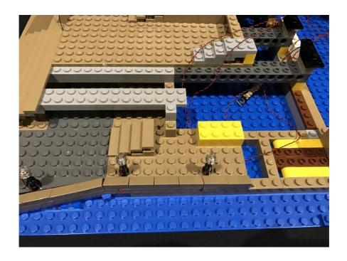
Connect the two lamp post cables to the expansion board.
