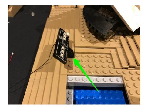
Loop the cable behind the spot light and then pull towards the inside. Thread the cable underneath the following section and then connect it to a spare port on the 12-port expansion board
