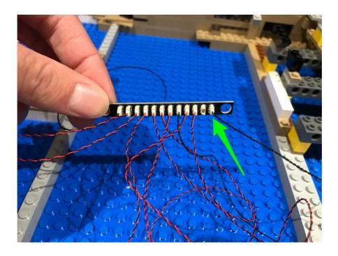
Connect the other end of the 30cm connecting cable to a **6-Port Expansion Board**
