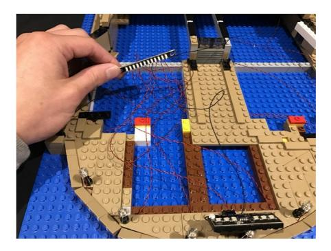
18.) Take the other end of the 30cm connecting cable closest to the top of the expansion board and thread it underneath the following section and then connect it to another **12-port Expansion Board**.
