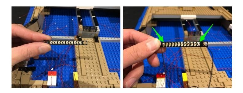
Take all the lamp post cables laid on the left side of the set as well as the 30cm cable from the spot light (there should be 10 in total) and connect them to the 12-port expansion board.
