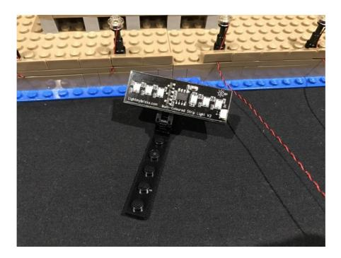
Take a **30cm Connecting Cable** and connect it to the port on the strip light. Connect the spot light to the following position on the set.
