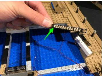
Connect the remaining 3 lamp post cables on the right side of the set to the next available ports on the expansion board.
