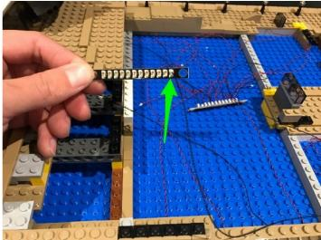
Connect the three lamp cables we have secured down, as well as the spot light cable to the expansion board.
