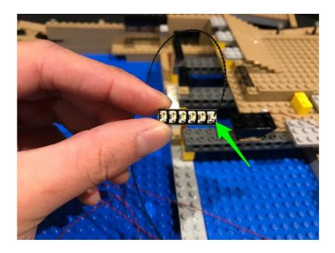
29.) Take the remaining three lamp post cables on the right and connect them to the 6-port expansion board. Reconnect the grey plate we removed earlier.
