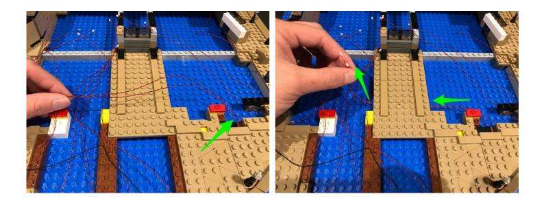
17.) Take a **12-port Expansion Board** and then take **2x 30cm Connecting Cables** and connect one to each port on the far sides.
