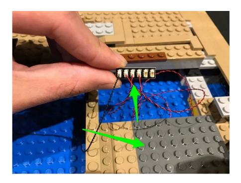
Take this time to test all the lights we have installed so far and to ensure everything is properly connected. To do so, take the **30cm USB Cable** and connect it to a spare port on the 6-port expansion board. Connect the other end to your USB power bank and ensure all lights are working OK.
