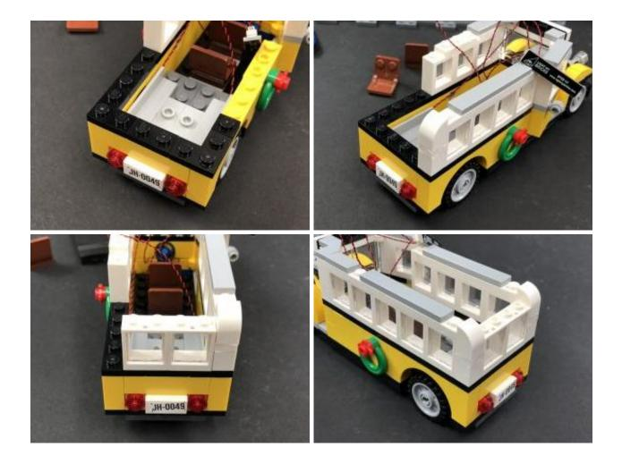
**8.)** Take the two tail light cables and connect them to the next spare ports on the Expansion Board, then turn ON the Flat Battery Pack to test the lights installed so far are working OK.
