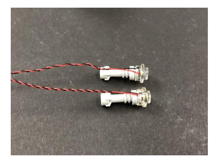
**2.)** Reconnect both headlights to the front of the bus ensuring the cable is on the bottom and in between each clip then lay each cable toward the inside of the bus in between the following studs.
