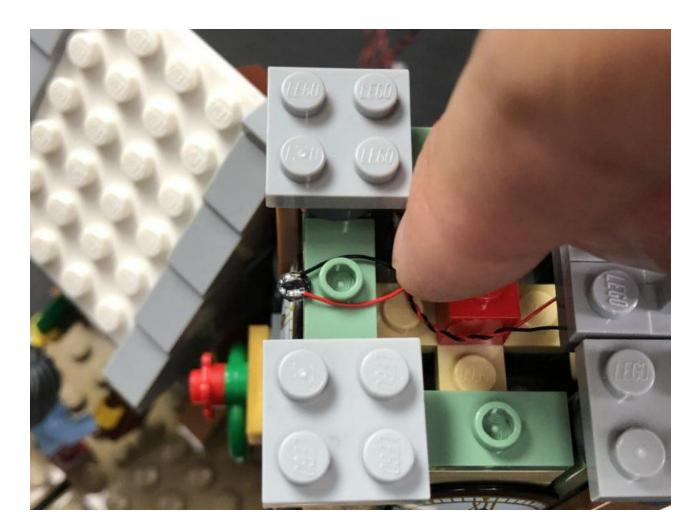
Secure the Bit Light in place by reconnecting the light grey section on the left side. The LED should be peeking out just above the clock on the left side to shine down.
