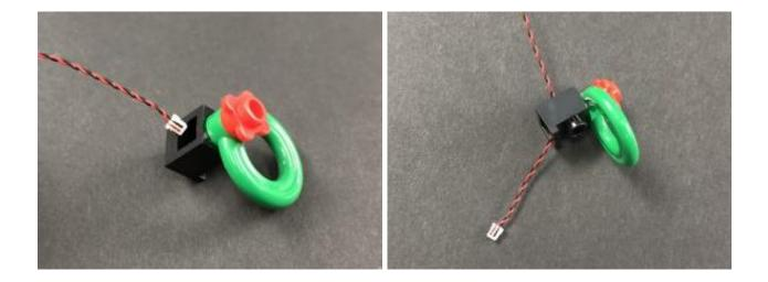
Pull the cable all the way through before reconnecting the lamp to the black brick ensuring the cable is facing the back.
