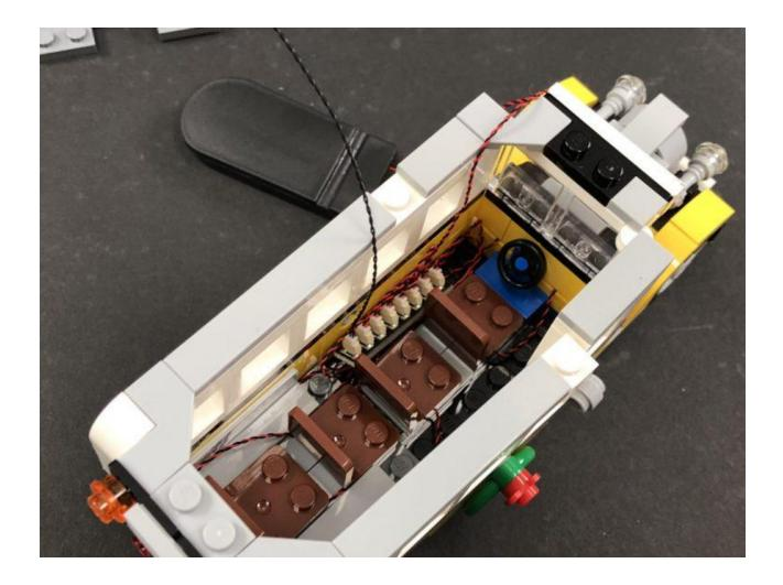
**14.)** Neatly place the battery pack down the right side of the bus ensuring the switch is facing the front.
