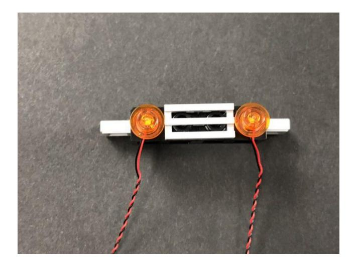
**10.)** Reconnect the upper rear light section to the back of the bus ensuring the cables are laid inside, then connect both cables to the Expansion Board.
