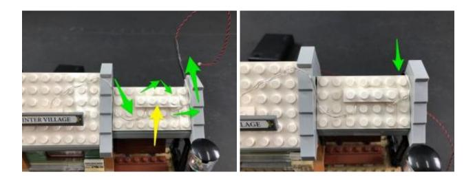
From the other side, bring the cable down and wind it around the black pole a few times before connecting it up to a spare port on the 12-Port Expansion Board.
