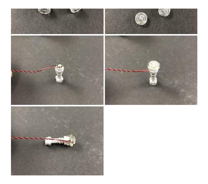
Repeat this process to install another **White 15cm Bit Light** to the other headlight, securing it in place using another provided **Trans Clear Round Plate 1×1.**
