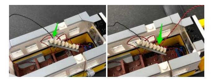
Neatly tuck all cables and expansion board in to the left side of the bus as per below (leave the other end of the 15cm cable out)
