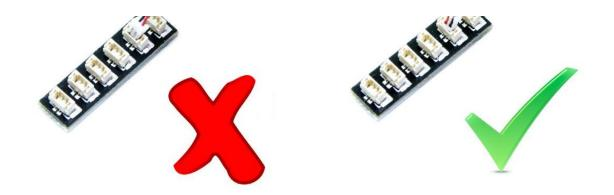
Incorrectly inserting the connector can can result in bent pins inside the port or possible overheating of the expansion board when connected.
