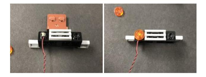
Repeat this step the install another **White 15cm Bit Light** to the other upper rear light securing it in place using another provided **Trans Orange Round Plate 1×1.**
