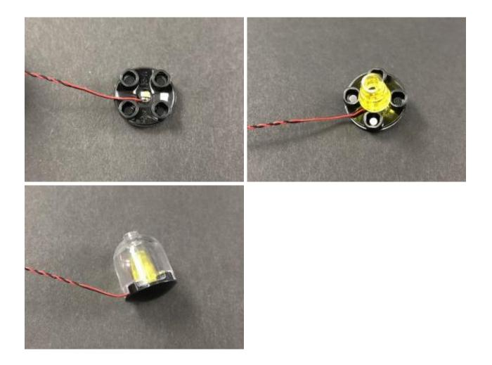
Thread the connector end of the cable through the top of the black brick and then pull it out from the back as shown below:
