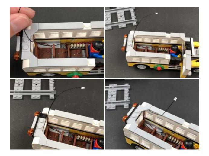
Take the roof of the bus and connect the cable to the Strip Light before securely reconnecting on top.
