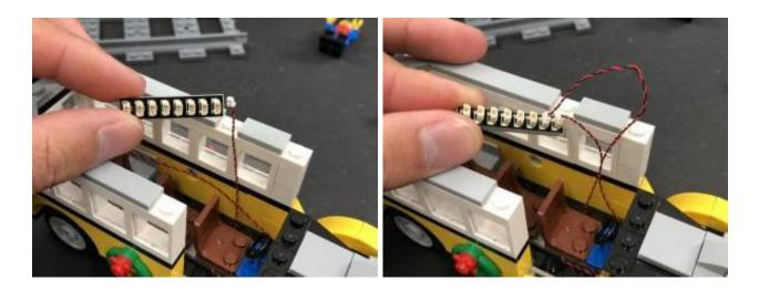
**4.)** Test the headlights by taking the **Flat Battery Pack** and inserting 2x CR2032 Batteries to it. Connect the battery pack cable to the expansion board and turn ON the battery pack to verify the headlights are working OK.
