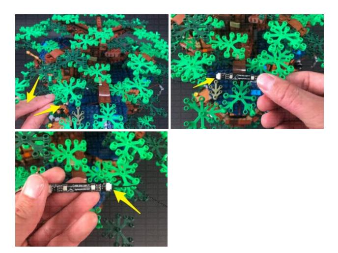
Stick the strip light on top of the back tree branch behind the dark brown curved plate as shown below, then secure the 15cm connecting cable on the left side in between the light green leaf spaces. Ensure the branch and leaf sections above are positioned over the strip light as much as possible.
