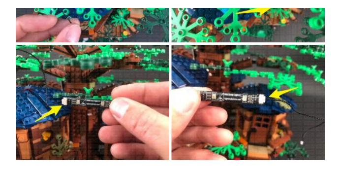
Using it's adhesive backing, stick the Strip Light across the top of the following two leaf pieces (dark green and light green underneath a larger tree branch). Ensure the leaf sections above are positioned over the strip light as per below
