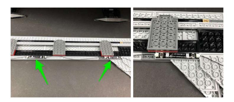
Mount the fourth strip light in the following position and then ensure all cables in between strip lights are tucked upward.
