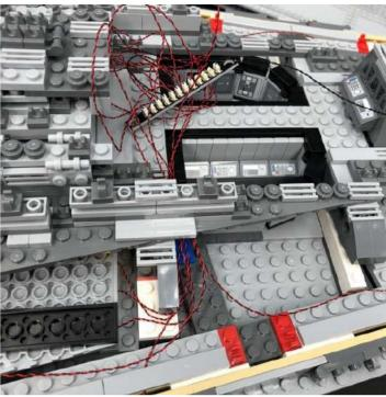
**27.)** Take the four remaining blue bit light cables toward the top right side of the ship and connect them to the next ports along on the 12-port expansion board above.
