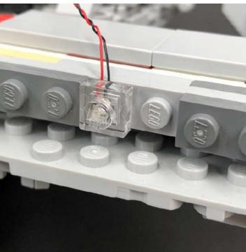
Hide the cable by laying it underneath the following 2x4 tile ensuring the cable is laid in between studs.
