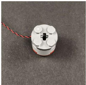
Reconnect this piece by pushing it back onto the technic bar. Do this very carefully to ensure the cable does not break. Reconnect surrounding pieces we removed earlier
