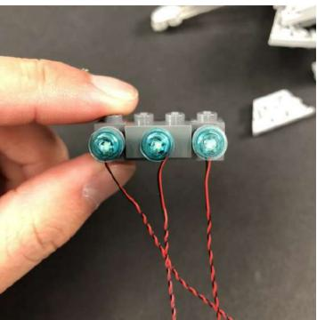
Reconnect the 1x4 brick to the small star destroyer, then reconnect the remaining piece ensuring the cables are laid in between studs.
