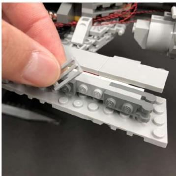
Take a **Blue 30cm Bit Light** and with the cable facing up, place it over the left stud as per below. Secure it in place by connecting a **provided LEGO Trans Clear Plate 1x1** over the top.
