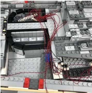
**35.)** Connect the two cables to a **6-Port Expansion Board.** Take another **15cm Connecting Cable** and connect it to the far end port on the expansion board.
