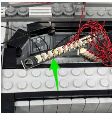
Lay all cables neatly along the back side of the control room (right side) and then reconnect sections we removed earlier over the top.
