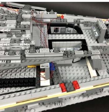
**18.)** Take another **8-Port Expansion Board** and connect all six cables to it (three cables from each side jet section)
