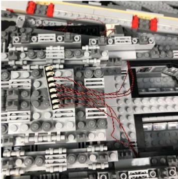
Take a **15cm Connecting Cable** and connect it to a spare port on the expansion board.
