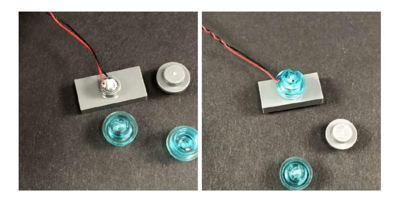
Install the remaining **Cool White 30cm Bit Light** to the other dark grey round plate and secure it in place by reconnecting the trans light blue plate over the top
