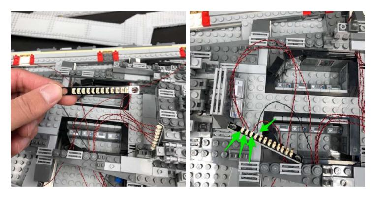
Take a **50cm Connecting Cable** and connect it to the far left port on the 12-port expansion board. Bring the cable toward the top of the ship and then connect it to the end port of a new **12-Port Expansion Board.**
