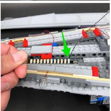
**24.)** Take the remaining four blue bit light cables toward the top of the ship and connect them to the 12-Port Expansion Board near by.
