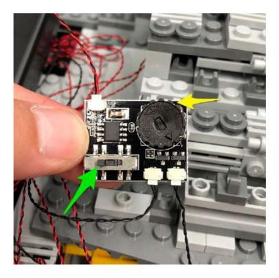
Once you have confirmed all is working OK and you are happy with your chosen effect, disconnect the battery pack cable and connect a **15cm Connecting Cable** to the IN port instead. Leave the other end of the cable disconnected for now.
