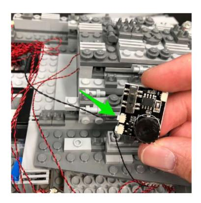
**19.)** Take the AA Battery Pack and insert 3x AA batteries to it. Place the battery pack on top of the ship and connect the battery pack cable to the IN port on the multi effects board. Turn the battery pack ON to test all jet lights are working OK.
