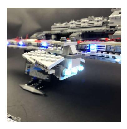
**40.)** Take the roof of the control room area we removed earlier and then push the AA battery pack into the space underneath ensuring the ON/OFF switch is accessible. Neaten up cables underneath before securely reconnecting the roof back on top of the control room.
