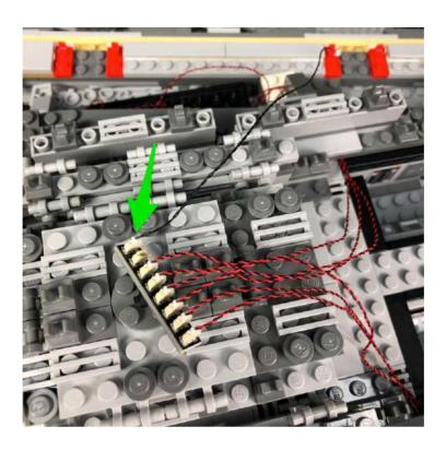
Turn the ship back around to the left side and then connect the other end of the 15cm connecting cable to the other OUT port on the Multi Effects Board.
