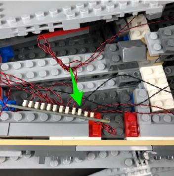
**44.)** Take the entire left roof section bring it over the top of the star destroyer. Take the other end of the 15cm connecting cable from the first blue strip light and connect it to a spare port on the 12-port expansion board underneath.
