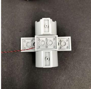
**7.)** Reconnect the three jets together then group the three cables and thread them inside the space behind before reconnecting to the main jet section.
