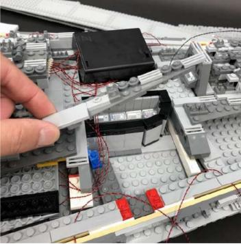
Take the back three blue bit light cables and connect them to the 12-Port Expansion Board near the control room area.
