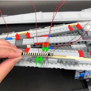
Take the AA Battery pack and connect the battery pack cable to the 12-port Expansion Board. Turn the battery pack ON to test all the blue lights are working OK. They should be illuminated along with the back jet lights however, they should be static (steady ON).
