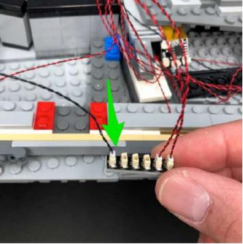
Connect the other end of the 15cm connecting cable to a spare port on the 12-Port Expansion Board in the control room area.
