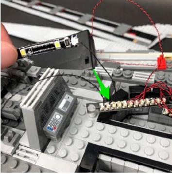
Using the strip light's adhesive backing, stick the strip light down on the the floor of the control room toward the front area as per below
