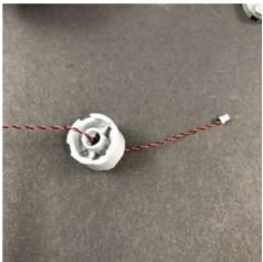
Slightly bend the Bit Light so that it is directly facing upward before pushing it down and reconnecting the trans orange plate over the top.
