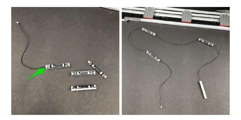
Using the adhesive backing on the end strip light, stick it down toward the right side of the roof section in the following position. Ensure the other components are on the left side.
