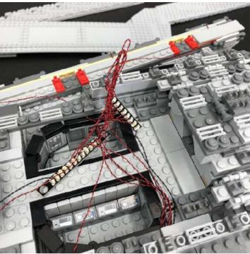
**30.)** Take a **White Strip Light** and connect a **5cm Connecting Cable** to one side. Connect the other end of the connecting cable to a spare port on the 12-port expansion board in the control room area.
