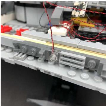
Hide the cable underneath the following tile ensuring the cable is laid in between studs.
