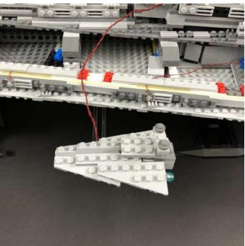
**39.)** Bring the cables over toward the back and then connect all three to the 6-port Expansion Board from step 35.
