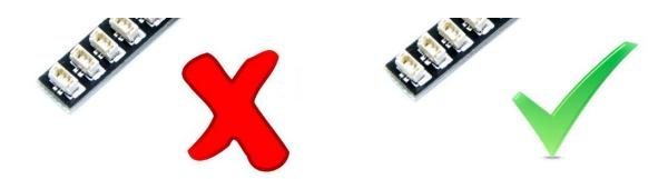
Incorrectly inserting the connector can can result in bent pins inside the port or possible overheating of the expansion board when connected.
