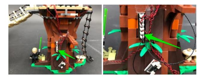
**38.)** Mount the Flicker Effects Board to the back of the tree using an **Adhesive Square.**
