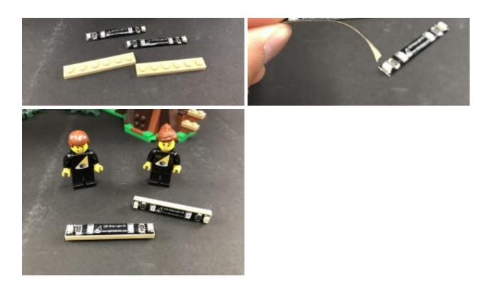
Connect the two strip lights together using a **15cm Connecting Cable** then take another **15cm Connecting Cable** and connect it to the right strip light's other port.
