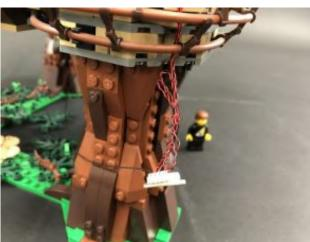
**13.)** Take a **50cm Connecting Cable** and connect it to the 6-port expansion board. Bring the cable around to the front and thread it through the bottom of the tree platform, then pull it all the way out as shown below:
