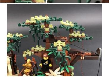
**7.)** Turn the village around the back and group all four green bit light cables together on the right side. Connect the lights to the 8-Port Expansion Board below, then turn the USB Power Bank ON to test the green tree lights are working OK.
