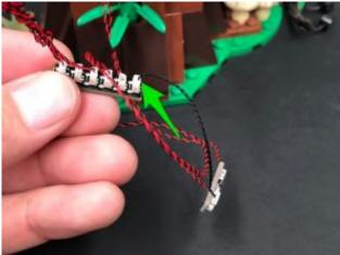
Using **2x Adhesive Squares**, stick the 6-port Expansion Board to the back of the tree in the below position:
