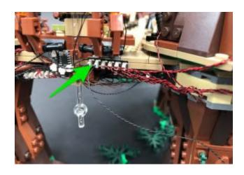
Hide the 30cm connecting cable underneath the tree platforms, then stick the 2-port Expansion Board underneath the tree platform on the right using another **2x Adhesive Squares.**
