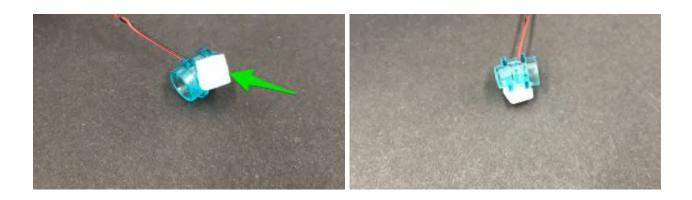
Mount the LEGO plates with Bit Light to the base of the bottle as shown below, then thread the connector end of the cable through the lower gap of the bottle. Pull the cable all the way out from behind.
