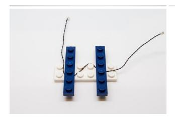
CAUTION: Forcing LEGO® to connect over a cable can result in damaging the cable and light.
