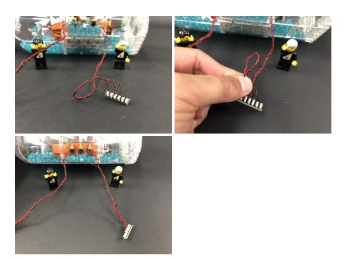
**13.)** Take a **Multi Effects Board** and connect a **5cm Connecting Cable** into one of the OUT ports (side with two ports). Connect the other end of the 5cm Connecting Cable to a spare port on the 8-Port Expansion Board.
