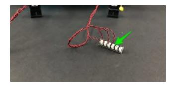
Twist/wind any remaining excess cables around the larger group of cables as shown below:
