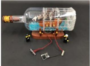
Twist/wind the two larger cables together then fold up the cables so they can be neatly hidden underneath the bottle in between the stand and bottle.
