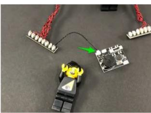
Take another **5cm Connecting Cable** and connect it to the IN port on the Multi Effects Board (side with one port). Connect the other end of the 5cm Connecting Cable to a spare port on the 6-Port Expansion Board, then connect the AA Battery Pack to the remaining Port.
