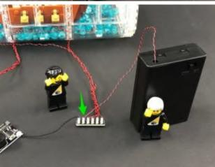
14.) We can now set the effect we want. For a slow effect to represent 'waves of the sea', we chose to the 'Pulse' effect. Flick the switch to the far right for 'Pulse', then turn the speed wheel all the way to the left for the slowest speed.
