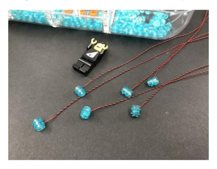
Take the **8-Port Expansion Board** and connect the AA Battery Pack to it, then connect all six Blue Bit Light cables. Turn ON the battery pack to test all the blue lights are working OK.
