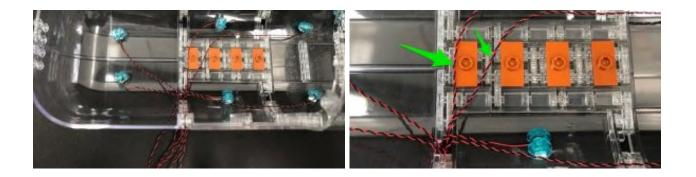
Twist/wind the six cables around each other all the way to the ends so they come together to form one larger cable, then starting with the shorter two cables, connect all six cables to the 8-Port Expansion Board.
