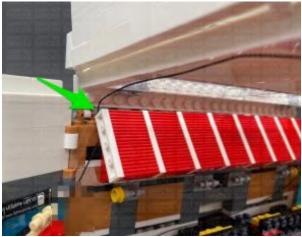
Connect the 30cm Connecting Cable to the next available port on the 8-Port Expansion Board.
