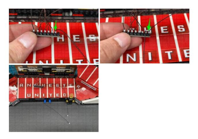
Take the other end of one of the 15cm cables and connect it to a **Blue Strip Light**. Connect another **5cm Connecting Cable** to the strip light's other port, then connect the other end of the 5cm cable to another **Blue Strip Light**.
