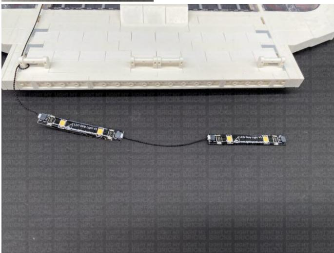
Take a **15cm Connecting Cable** and connect it to the white strip light's right port, then using the adhesive backing on the strip lights, stick both of them underneath the roof to the following positions.
