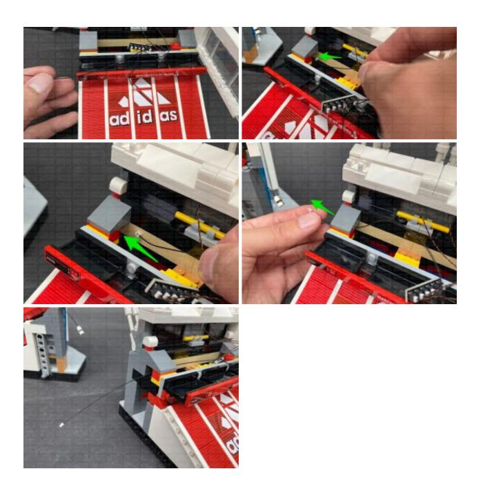
**25.)** Take the spare 5cm cable from the expansion board and connect it to the right port on a new **White Strip Light**. Take a **15cm Connecting Cable** and connect it to the strip light's other port.
