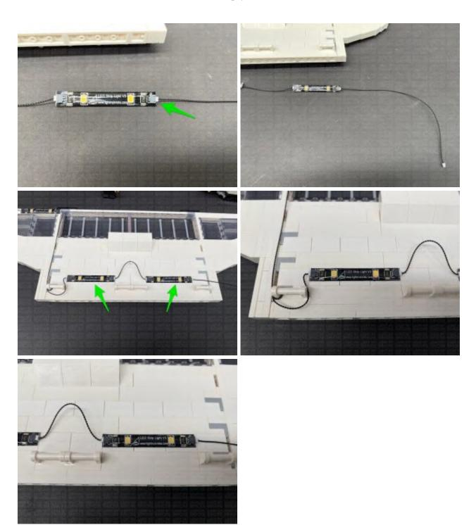
**31.)** Bring the 15cm cable over the right side of the white handle, then thread it up through the space underneath. Pull the cable out from the top, then thread it through the handle again to create a double loop.
