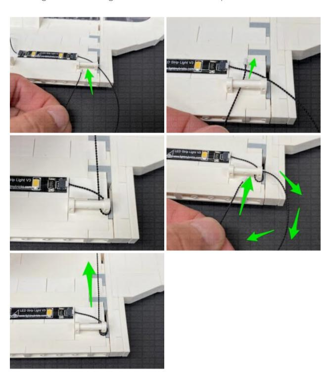
Connect the other end of the 15cm cable to the remaining **White Strip Light**, then using it's adhesive backing, stick the strip light underneath the roof to the following position.
