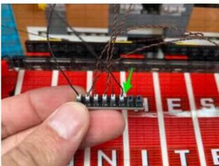
**16.)** Take **2x 15cm Connecting Cables** and connect them to the two remaining ports on the expansion board.
