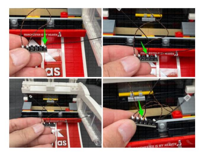
right. Pull the cable out from the other side (East Stand) and connect it to a **2- Port Expansion Board.**
