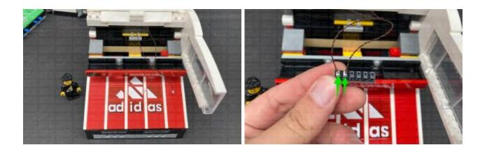
Take 2x 5cm Connecting Cables and a 15cm Connecting Cable, and connect them all to spare ports on the 6-Port Expansion Board. Ensure you connect one of the 5cm cables to the far right port on the expansion board.
