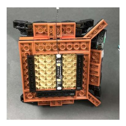
**18.)** Take the roof above the third floor and connect the other end of the 5cm connecting cable to a spare port on the 6-port expansion board underneath before securely reconnecting the roof.
