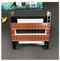
29.) Take a White Strip Light and stick it to a provided LEGO Plate1x6. Take a 30cm Connecting Cable and connect one end to the Strip Light.
