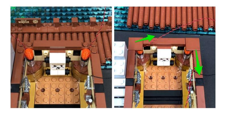
**36.)** Take an **8-Port Expansion Board** and connect all four bit light cables as well as 15cm cable from underneath to it
