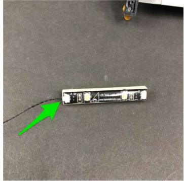
Mount the Strip Light underneath the roof in the below position ensuring the cable is facing the left side as per below.
