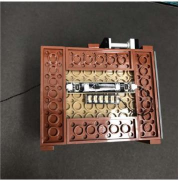
Take the **AA Battery Pack** and insert 3x AA batteries to it. Connect the Battery Pack cable to the 6-port expansion board as per below.
