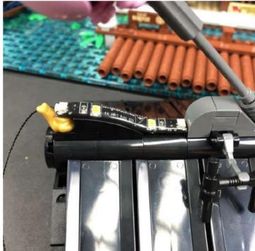
Pull the cable down the side and secure it underneath the black round tile with hole.
