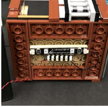
**4.)** Take another **15cm Connecting Cable** and connect it to one of the ports on the 6-port Expansion Board. Lay the cable underneath the right 2x8 plate ensuring it is laid in between studs.
