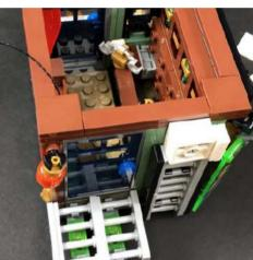
**12.)** Take the third floor and place it over the second floor. Take the 15cm connecting cable from the left side underneath the brown tile and connect it to the 6-port expansion board below.
