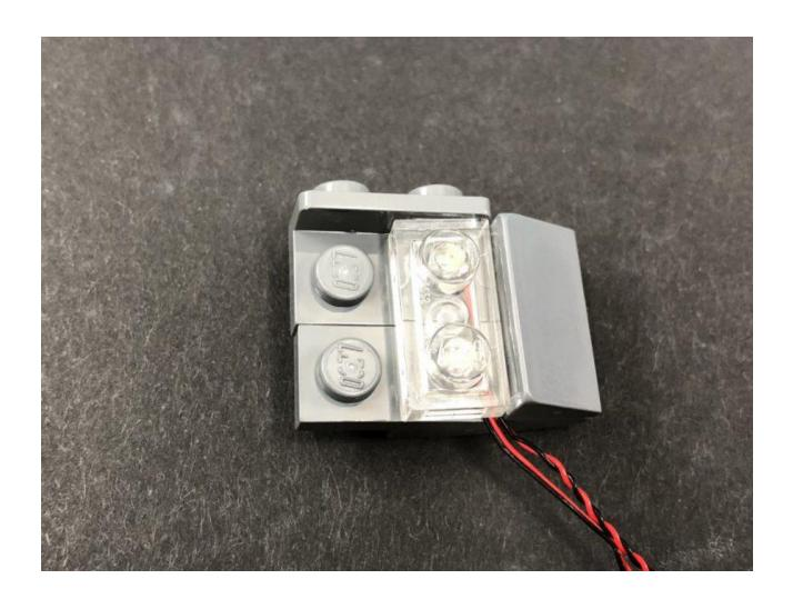
Take another **2x Cool White 30cm Bit Lights** and position them together the same way as we did the previous two bit lights. Place them over the top of the two left studs of the headlight section as shown below and then secure them in place by reconnecting the trans orange 1×2 plate over the top. Ensure both Bit Lights are comfortably siting in the inside of each trans orange stud.
