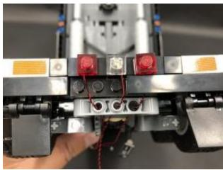
Ensure the first and second cable is neatly laid in between studs before reconnecting the registration plate over the top.
