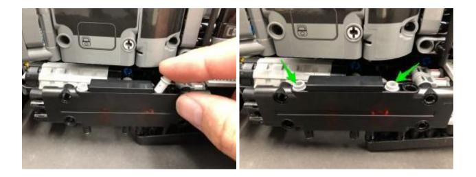
Take a **White 15cm Bit Light** and thread the connector end of the cable down the holes of one of the technic pins we just connected. Thread it all the way through (ensuring it does not go through the second hole on the back of this section) then secure it in place by reconnecting the trans orange plate over the top this time, with the stud facing up.
