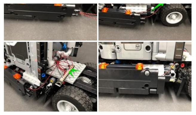
Reconnect the Battery Pack Cable to a spare port and verify the left side lights are working OK.
