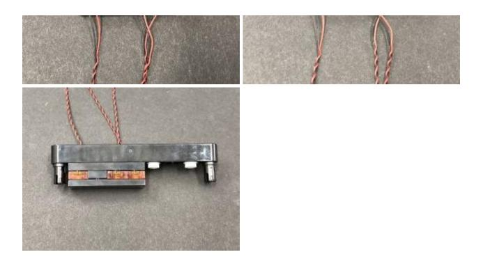
13.) Disassemble the right section and then repeat the previous step to install another 2x White 30cm Bit Lights.
