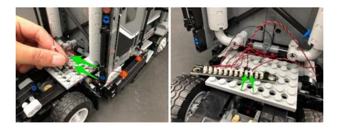
Reconnect the panel section then connect the battery pack cable again and test the side lights are working OK.
