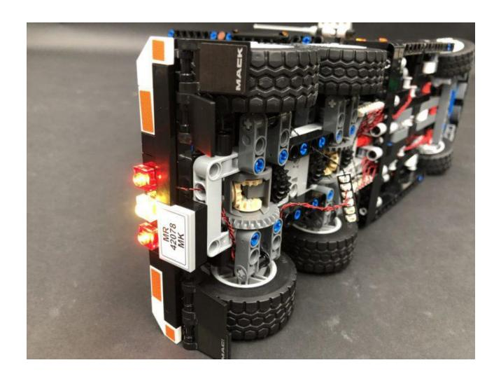
**24.)** Take **2x Adhesive Squares** and stick them to the back of the 6-port expansion board. Mount the expansion board underneath the truck in the following position. Ensure the expansion board is clear from the turning gears, then push the cable down and out of the way.
