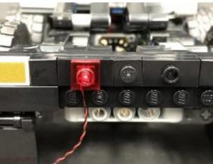
Take another **White 15cm Bit Light** and place it over the next stud along. Secure the bit light in place by connecting a provided **Trans Clear Plate 1×1** over the top.
