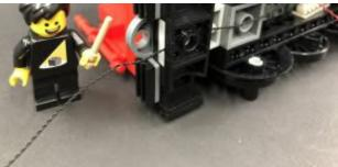
Twist and fold excess cabling from underneath the train, then tuck them in neatly to prevent them from dangling down. Bring the other 15cm connecting cable toward the back and pull it up the left side of the train as shown below:
