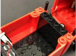
**26.)** Take another **15cm Connecting Cable** and connect it to the 6-port Expansion Board. Disconnect the back wall, then pull the other end of the cable all the way out the back. Reconnect the back wall over the top ensuring the cable is in between studs.
