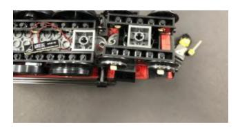
Take a **Round Battery Pack** and insert 2x CR2032 Batteries to it. Connect the battery pack to the 6-port expansion board and turn it ON to test the lights on the front of the train are working OK.
