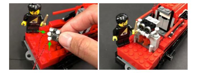
Eliminate excess cables by twisting/folding the bit light cables around each other so they come together in a neat bunch, then tuck them (along with the effects board) inside.
