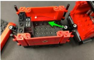
Reconnect the connecting cable to the 6-port expansion board from previous step, then reconnect the front wall over the cable ensuring the cable is laid in between studs and that there is enough cable slack for the carriage to turn left/right.
