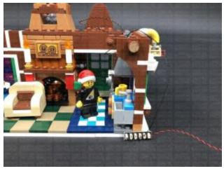
Disconnect the following brown 1×1 brick at the top, then bring the 15cm Connecting Cable over the left arched brick and lay it in between studs as shown below. Ensure there is just enough cable length from the top and the expansion board, then reconnect the brick over the top. Pull any excess of the 15cm cable from the inside up so that it doesn't dangle down.
