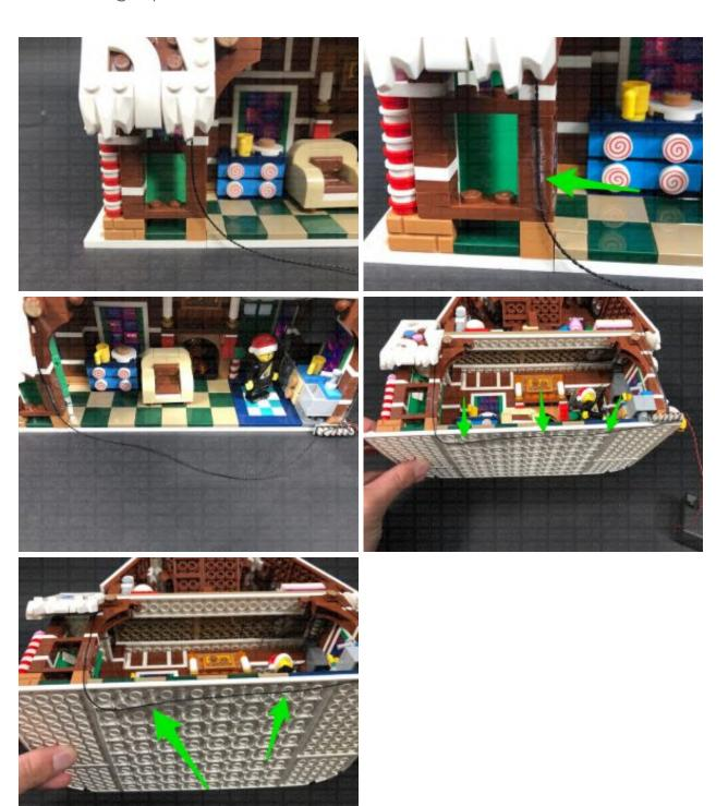
**39.)** Position the Christmas Tree next to the Gingerbread House, then take the 30cm Connecting Cable from the bottom of the tree and connect it to a spare port on the 8-Port Expansion Board on the right side of the House.
