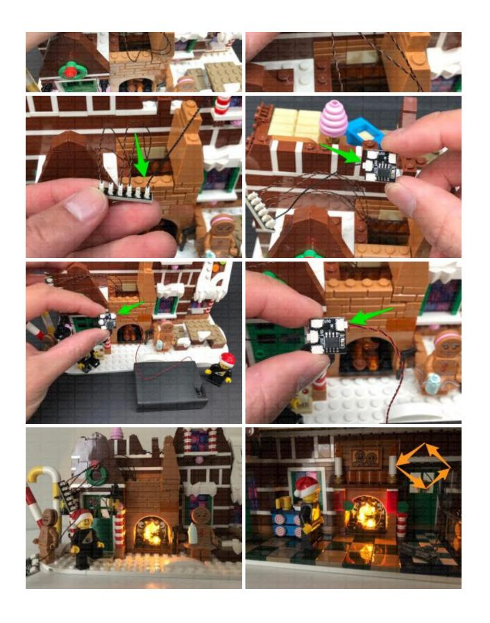
Note: If you experience any issues with the lights not working and suspect an issue with a component, please try a different port on the expansion board to verify where the fault lies (with the light or expansion board). To correct any issues with expansion board ports, please view the section addressing expansion board issues on our **online troubleshooting guide.**
