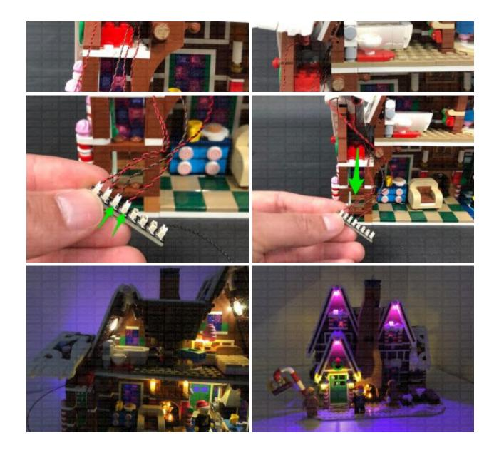
**36.)** We will now install the remaining light to the left side of the bottom floor. Carefully turn the house over onto it's front then turn it upside down so we can access underneath the top floor. Take the remaining **White 15cm Bit Light** and with the cable facing the left and led facing up, place it underneath the top floor in the following position. Secure the Bit Light in place by connecting the remaining provided **Trans Clear Plate w Rounded Bottom 2×2** over the top of it.
