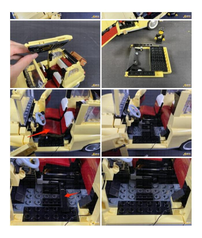
Take the remaining **White 15cm Bit Light** and connect the cable to the **OUT** port on the NC Push Board. Remove the protective backing on the NC Push Board, then using the adhesive underneath, stick the board to the floor of the vehicle near the edge of the door opening as shown below. Ensure the push trigger is facing out.
