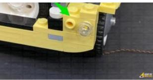
**3.)** Repeat the previous step to install another **White 15cm Bit Light** to the bottom right headlight, then reconnect this section to the front right side of the car.
