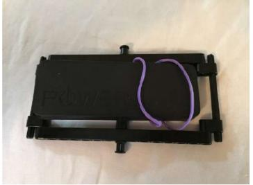
Put the rubber bands around the USB power bank and move them approximately one third of the way down the power bank. Sit the power bank on top of the centre section.
