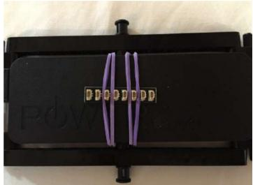
Grab the **8 port Expansion Board** and secure it to the power bank underneath the rubber bands.
