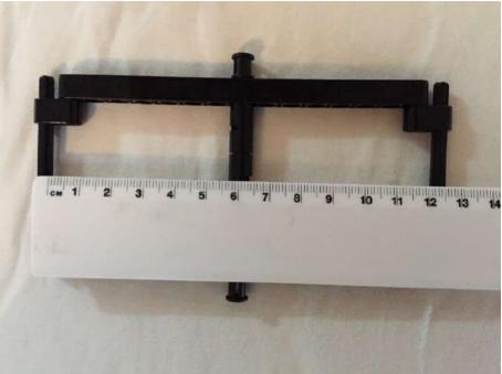
The USB power bank (Not included in this kit) will be attached to the centre section. Your power bank should be small enough to not exceed the length and width of the centre section which is approximately  $4.7 \, \text{cm} \times 12 \, \text{cm}$ .
