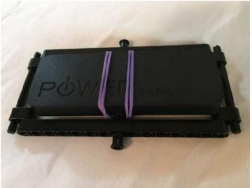
Pull the rubber bands underneath the middle of the centre section where the round technic pin connectors are.
