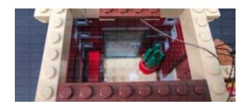
**34.)** Secure the 15cm Cable from the left side of the building underneath the side 1×10 plate, then take a new **15cm Connecting Cable** and connect it to the other large port on the Micro Expansion Board.
