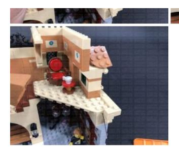
Bring the 30cm Cable up to the top floor and lay it around the following studs, then reconnect the brown angled bricks over the top. Bring the cable up to the top of the set and connect it to a new **Micro 4-Port Expansion Board** (large port).
