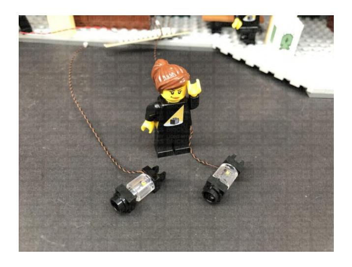
10.) Thread each of the lamp cables through the gaps on the pillars. Pull the cables all the way out from behind before reconnecting the lamps. Bring both cables towards the 12-port expansion board.
