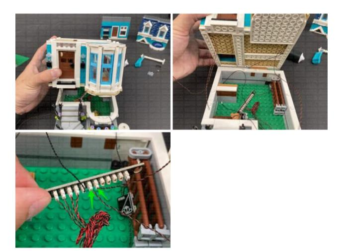
Connect the Wireless Connector and the other end of the 5cm Connecting Cable from the flicker effects board to the 12-port Expansion Board.
