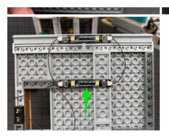
Secure the wireless connector cable by laying it in between studs and connecting a provided LEGO **Plate 1×6** over the top. Secure any remaining excess cable underneath the dark grey 1×10 plate.
