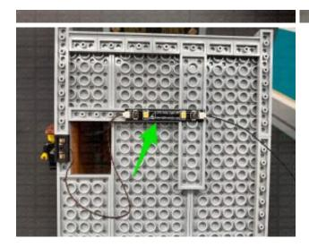
Secure the wireless connector cable by pushing it up inside the plate holes as shown below, then secure the cable by connecting a provided **Plate 1×6** over the top.
