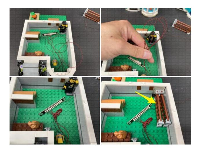
Take out the **50cm Connecting Cable** and connect it to a spare port on the expansion board, then thread it through the technic brick hole that leads to the outside of the building (left side). Pull the cable all the way out from the outside. This cable will be used to connect up to the left building (book shop).
