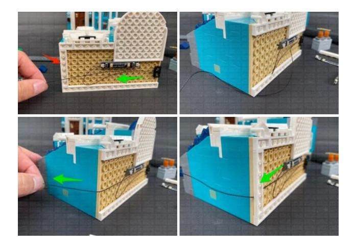
Tuck in any excess cable from the wireless connector to prevent it from dangling down.
