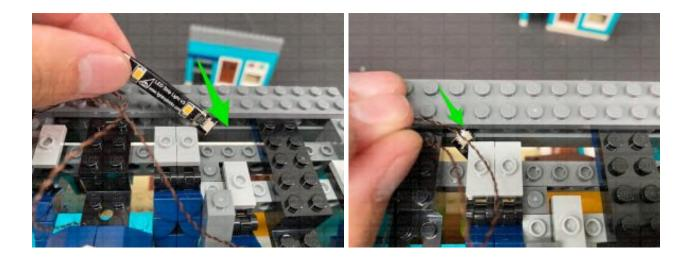
Take the top floor and securely place it over the rest of the building. Ensure that both wireless connector contacts are aligned and touching each other. Turn ON the power to test the lights to the top floor are working OK. The lights will deactivate when the top floor is removed. It will activate when the top floor is reconnected as long as the wireless connector contacts are aligned.
