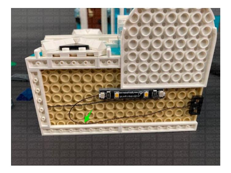
**13.)** Turn the top floor back over and pull the 30cm Connecting Cable up the left side of the building. Connect it to a spare port on the 6-Port Expansion Board above.
