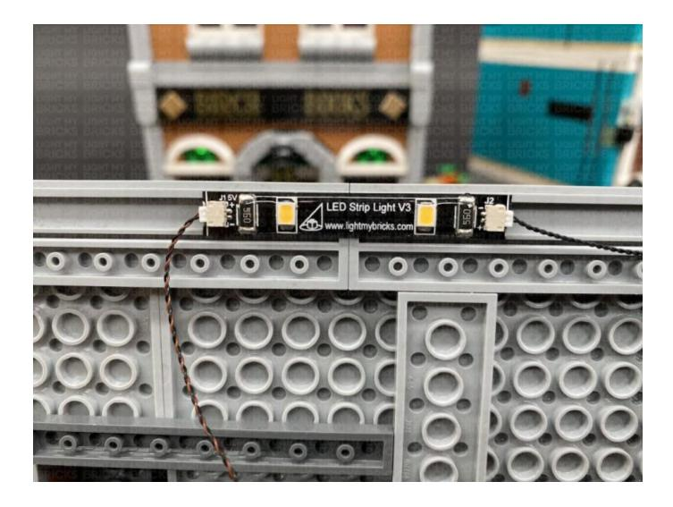
28.) Connect the other end of the 5cm Connecting Cable to a new Warm White Strip Light. Take the remaining 15cm Connecting Cable and connect it to the other end of the Strip Light, then using it's adhesive backing, stick this strip light to the following position underneath the top floor.
