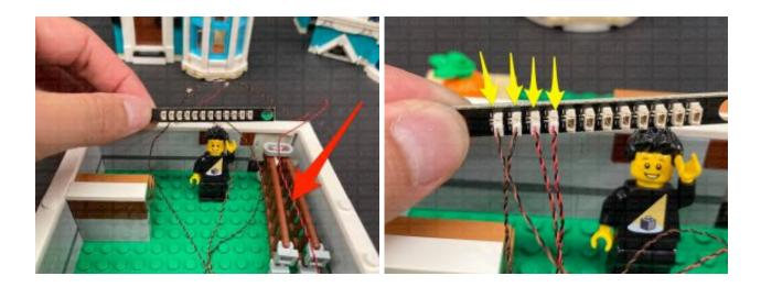
Take the **USB Power Cable** and thread the connector end of the cable through the technic brick hole on the outside of the building on the right side. Pull the cable in from the inside of the building, then connect it to the far right port on the expansion board. Connect the USB connection end to your **USB Power Bank** or **wall adaptor** (sold separately) and turn it ON to test the lamp post and garden lights are working OK.
