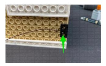
Take out a **Warm White Strip Light** and using it's adhesive backing, stick it to the base of a provided LEGO **Plate 1×6.** Connect the Wireless connector plug to the right port on the Strip Light. Take a **30cm Connecting Cable** and connect one end to the left port on the Strip Light.
