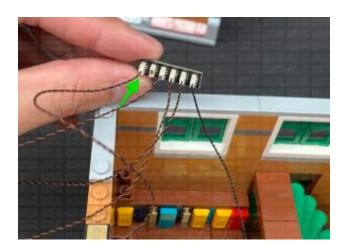
Group the three bit light cables together in between the following studs, then secure them down by reconnecting the 1×2 tile and longer 1×8 tile on both sides. Ensure the three cables are side by side and flat rather than over the top of each other.
