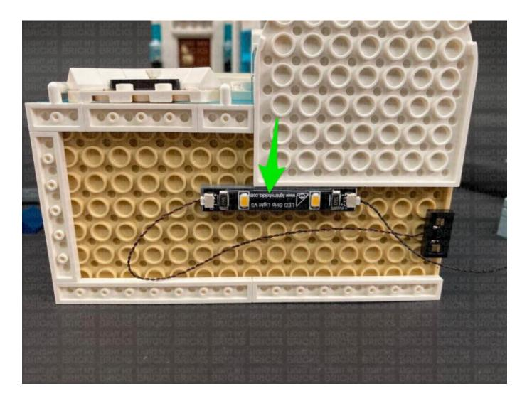
Bring the 30cm Connecting Cable across to the left side and over the wireless connector cable. Disconnect the white 1×6 plate from the left side and pull the 30cm cable up the wall. Reconnect the 1×6 plate ensuring the cable is laid in between studs.
