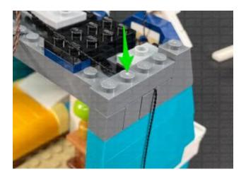
Disconnect the black 2×4 plate and lay the 30cm cable across and in between studs. Reconnect the black 2×4 plate, followed by the larger dark grey plate 2×16 plate.
