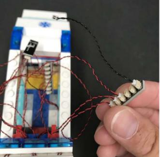
36.) Take the **Multi Effects Board** and then connect the remaining **5cm Connecting Cable** to the input port of the effects board (side with 1 port).
