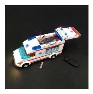
34.) We will now connect the 2 remaining lights from the top of the back door to the expansion boards where the front roof lights are connected to. Turn the ambulance to the backside and then take the bit light on the right side and connect it to the 6-port expansion board on the left side.
