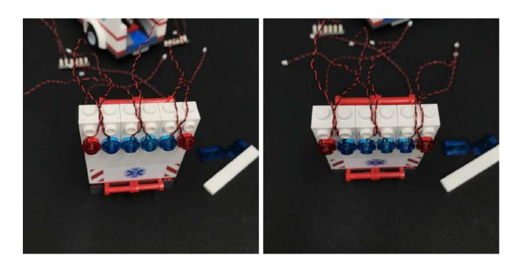
20.) Take the **provided LEGO Plate 1x6** and connect it over the top of the cables then reconnect the white 1x6 tile at the front.
