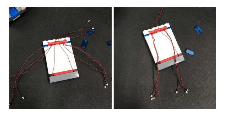
24.) Take the **8-port Expansion Board** and connect both groups of cables (Total of 6) to the spare ports.
