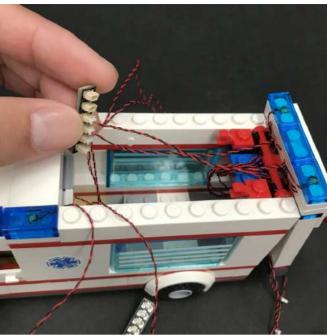
Locate the other end of the 5cm connecting cable from the 8-port expansion board and bring this back in and connect it to the 6-port expansion board inside (where the head and tail lights are connected to)
