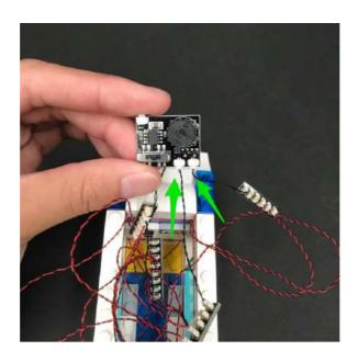
38.) Program the effects board by flicking the switch to the middle (emergency effect) and then turn the battery pack on to verify the effect of the roof lights. Turn the wheel on the effects board to adjust the speed of the flashing effect.
