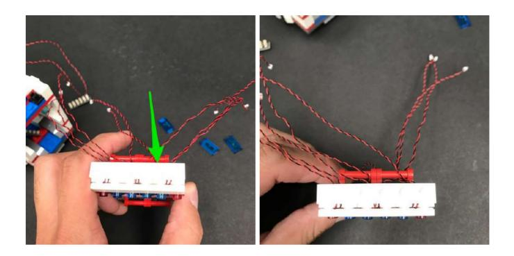
Repeat this step to thread down the three cables on the left, down the space of the other red 1x2 plate with handle.
