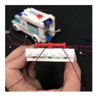
23.) Take each group of three cables which have been threaded down from the top and then twist them around each other forming one thicker cable for each side.
