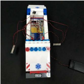
35.) Take the  $\bf 2x$  5cm Connecting Cables and connect each one to each of the 6-port expansion boards on each side.
