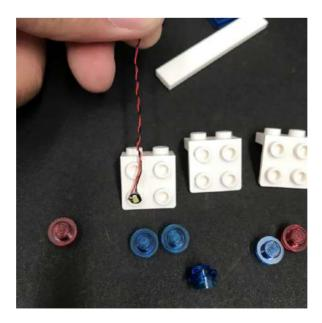
Secure the light in place by reconnecting the trans red plate over the top.
