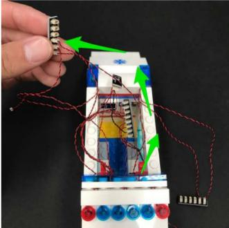
Take the bit light on the left side and connect it to the 6-port expansion board on the right side.
