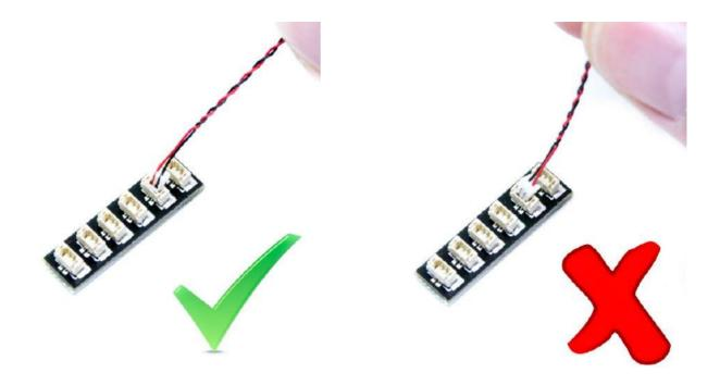
Incorrectly inserting the connector can can result in bent pins inside the port or possible overheating of the expansion board when connected.
