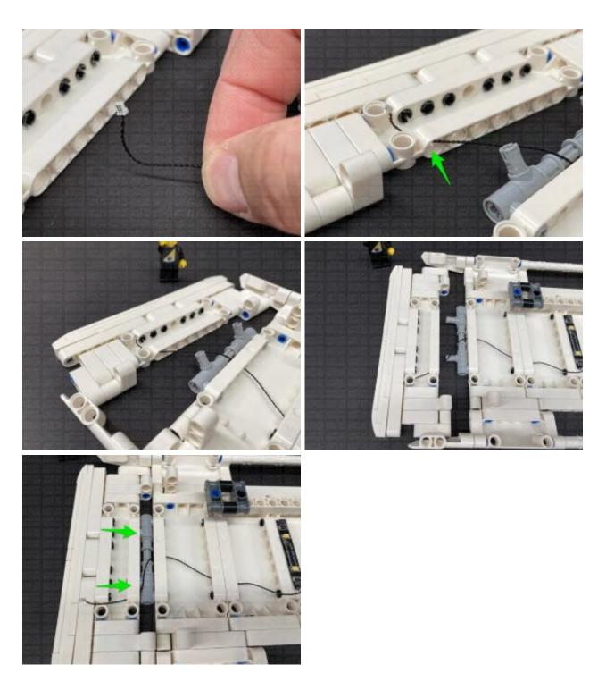
**15.)** Connect the cable to a new **White Strip Light**, then take a **30cm Connecting Cable** and connect it to the strip light's right port. Using it's adhesive backing, stick the strip light to the roof in the following position. Ensure the 30cm cable is facing up as shown below
