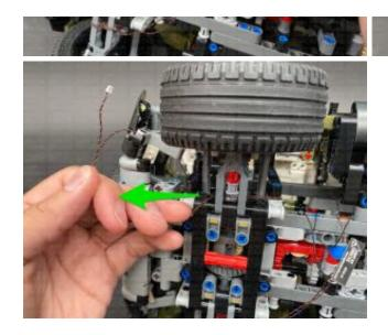
Thread the cables through the following technic hole, then loop it through the same hole again to secure and eliminate excess cabling. Connect the two cables to the 6-Port Expansion Board.
