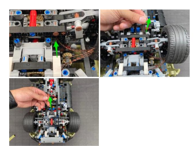
Turn the vehicle around to the side, and bring the cables back over and loop them around the wheel axis 3-4 times to eliminate excess cables, then connect them to the 12-Port Expansion Board
