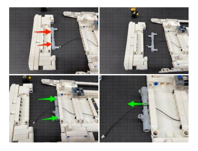
Fold the tip of the connecting cable into a "hook" shape, then hook the cable through the following hole on the technic pieces, then reconnect them to the grey technic pins, while pulling the cable out from the other side.
