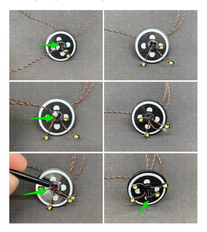
Reposition the 4 LEDs so they are evenly spaced out and positioned over the circles on the stickers behind, then reconnect the trans clear dish over the top. Reconnect the headlight to the rest of this section via the technic bar.
