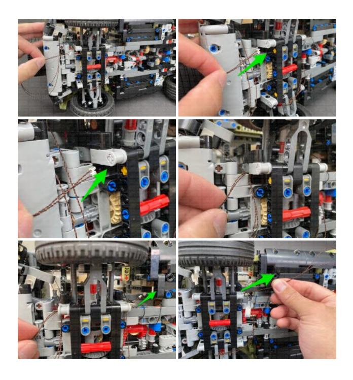
Thread the cables through the middle of the wheel axle, pulling it all the way out from the back side.
