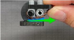
Bring this section over to the left side of the vehicle and thread the cables in between the two sections as shown below. Reconnect the headlight via the technic vertical axle.
