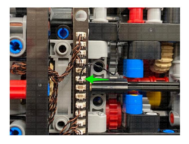
Take the AA Battery Pack and connect it to a spare port on the expansion board, then turn it ON to test the internal strip lights are working OK.
