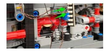
**26.)** Take **3x Adhesive Squares** and stick them to the back of the 6-Port Expansion Board. Mount the expansion board underneath the vehicle to the following position.
