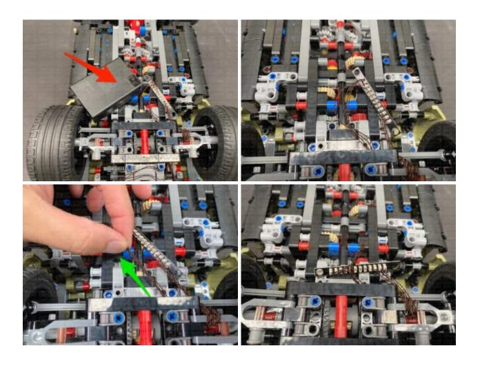
Turn the vehicle over to the side, then tuck the bunched up cables through one of the technic plate holes as shown below. Take **3x Adhesive Squares** and stick them to the back of the 12-port expansion board, then stick the expansion board to the following position.
