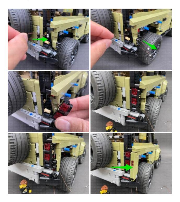
Turn the vehicle onto it's left side so that we can access underneath, then thread both Bit Light cables underneath the wheel axle as shown below. Pull the cables all the way out from the other side.
