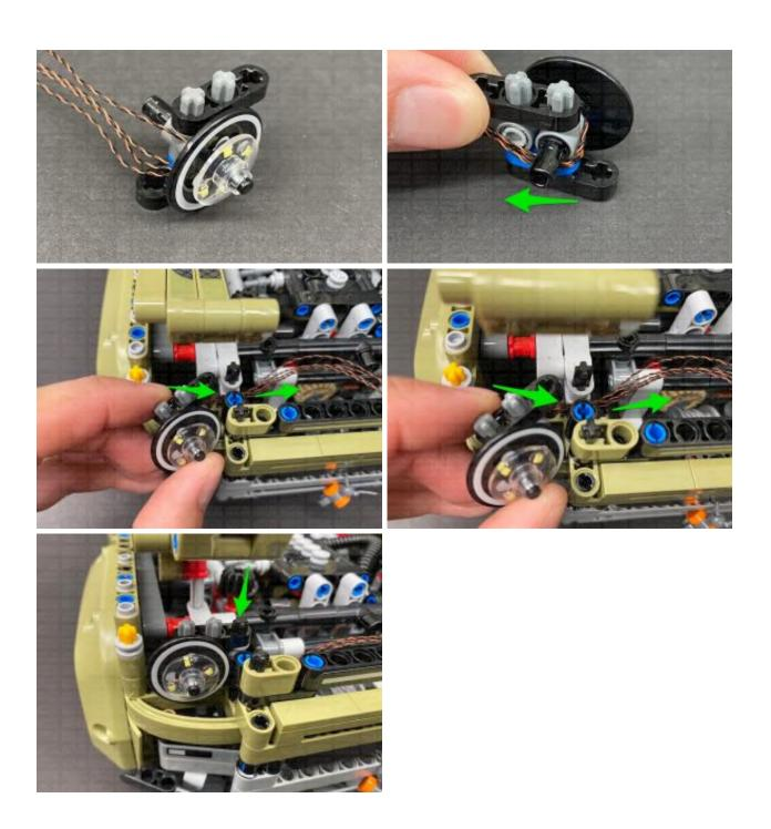
Group the 4 cables together and thread them down the following space behind the front grill. Prop the vehicle up using your light kit box, then pull the cables down from underneath as shown below.
