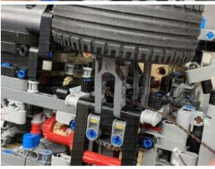
Thread the cables through the following technic hole in the axle. Loop the cables through a second time to secure and eliminate excess cabling. Connect both cables to the 6-Port Expansion Board, then turn the Battery Pack ON to test the tail lights are working OK.
