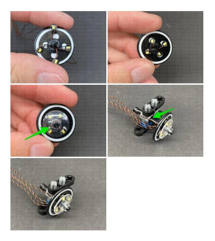
**4.)** Turn this section around and bring the 4 cables across to the right side underneath the technic pin. Bring this section over to the left side of the vehicle and thread the cables in between the two sections as shown below. Reconnect the headlight via the technic vertical axle.
