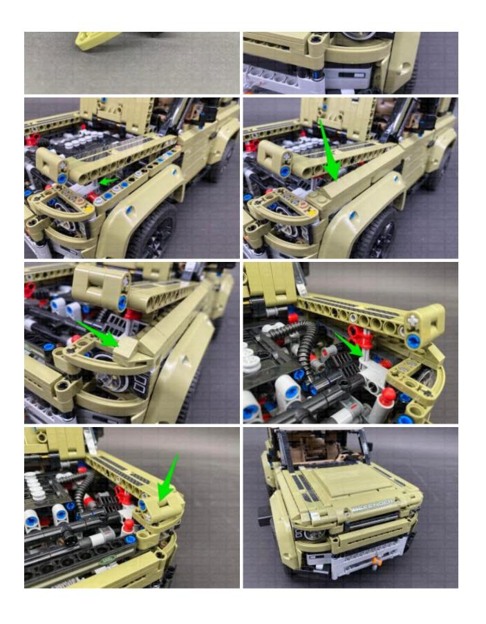
11.) Flip the vehicle back over again and disconnect the AA Battery Pack from the expansion board. Pull the four cables from the left headlight all the way out near the expansion board to eliminate any excess cable, then twist them
