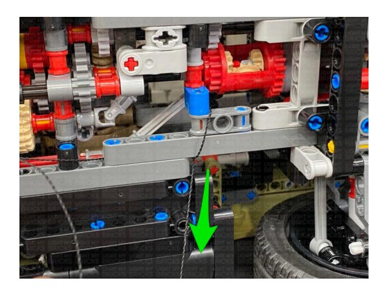
Loop the cable around these pieces a second time, then connect it to a **6-Port Expansion Board**.
