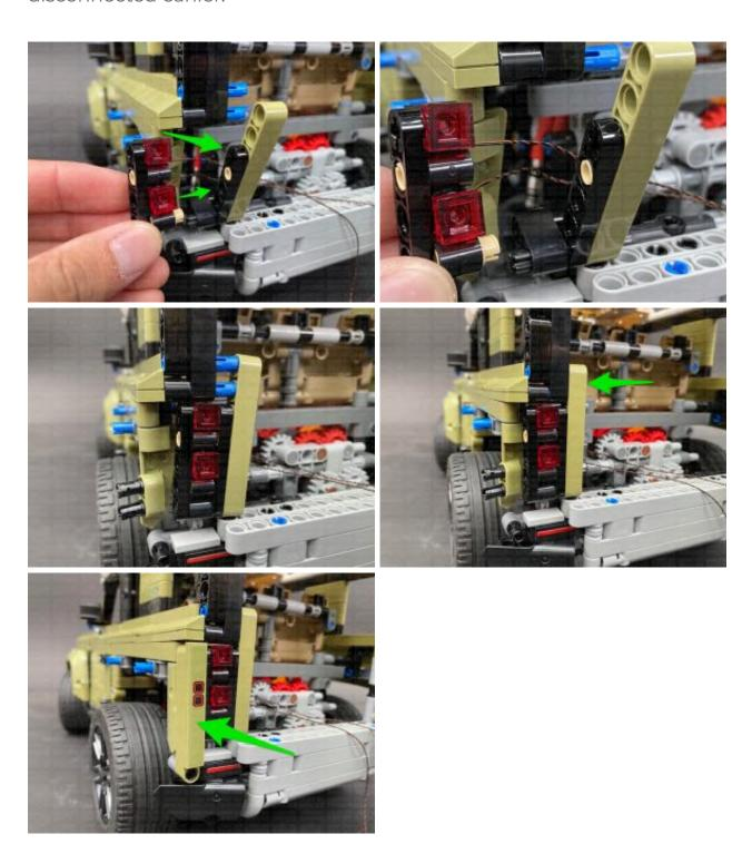
Pull out both Red Bit Light cables from behind the back wheel.
