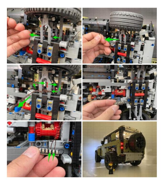
Note: If you experience any issues with the lights not working and suspect an issue with a component, please try a different port on the expansion board to verify where the fault lies (with the light, expansion board or effects board). To
