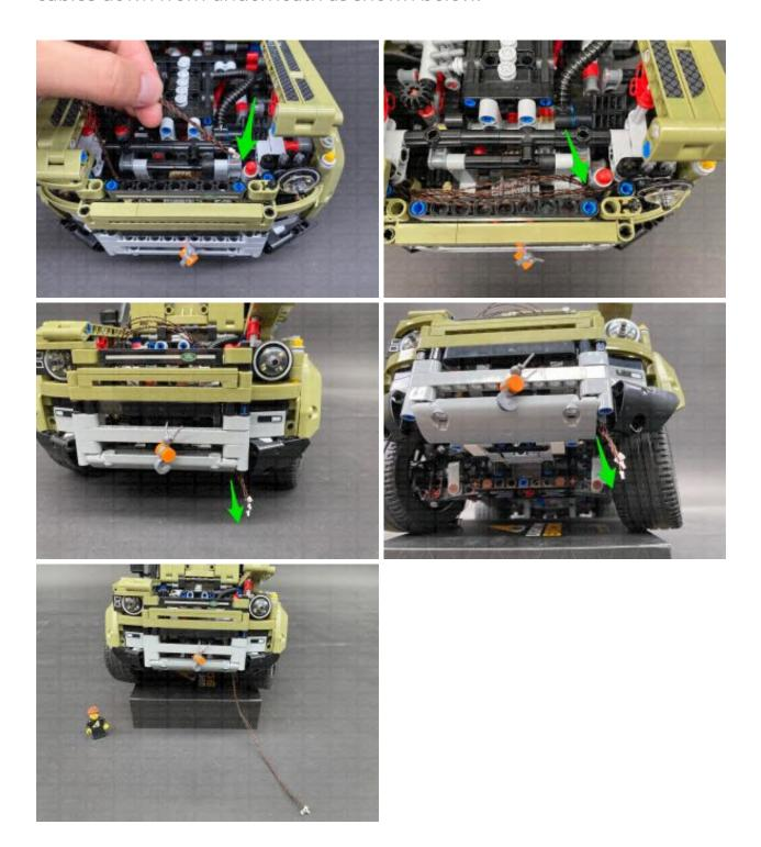
Flip the vehicle over and bring the four cables across to the right side, then thread them underneath the following technic pieces, pulling them all the way out from the other side.
