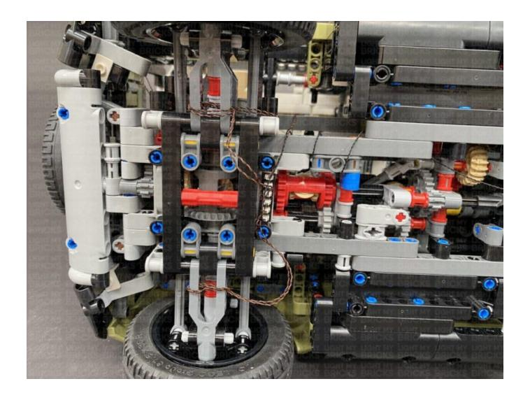
Eliminate any excess cables by twisting and folding them around each other into a neat bunch. Ensure that the wheels can still turn left and right.
