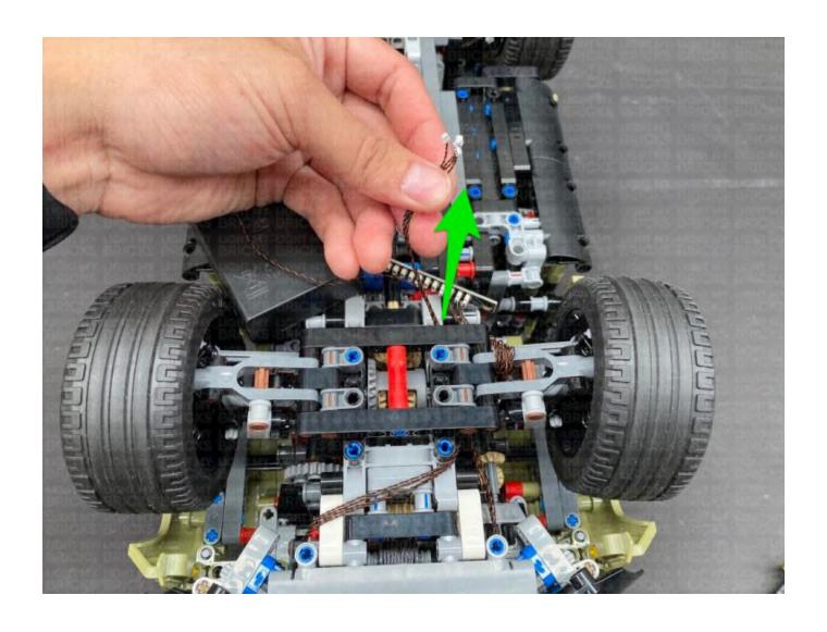
Ensure the cables are laid around the following section, then connect them to the left ports on the 12-port expansion board. Turn the power ON to test the left headlights are working OK.
