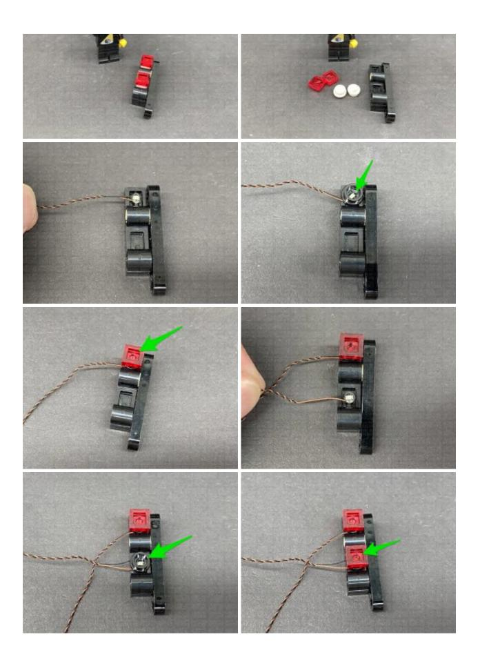
25.) Thread both Bit Light cables from the right tail light section through the
