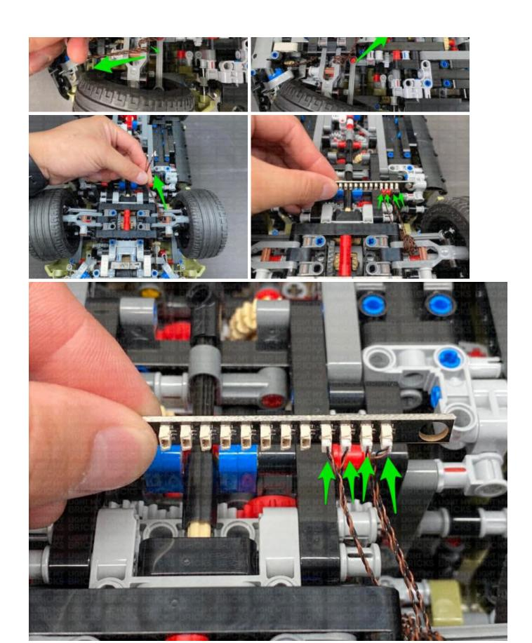
Take the **AA Battery Pack** and insert 3x new AA batteries to it. Connect the battery pack cable to a spare port on the 12-port expansion board then turn it
