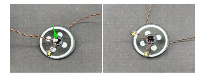
**3.)** Continue threading another 2x **Cool White 30cm Bit Lights** through the dish, then take LEGO Bar we removed earlier and insert it through the technic axle hole. Ensure the cables are laid in the technic axle spaces, to prevent them from being damaged when inserting the bar.
