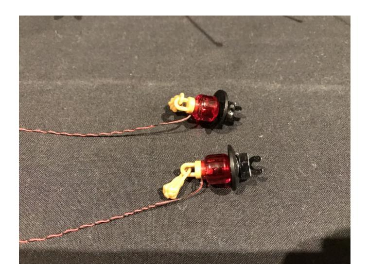
Take the cable from the bit light and then pull it up and then across the top and lay in between the black clip for both lanterns.
