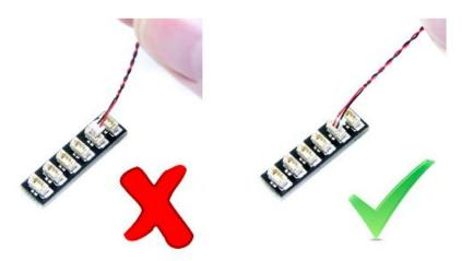
Incorrectly inserting the connector can can result in bent pins inside the port or possible overheating of the expansion board when connected.
