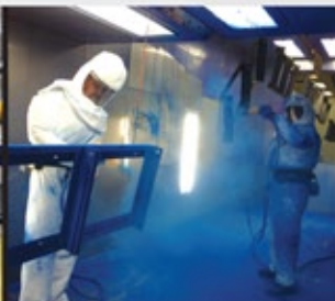
Powder Paint Line
