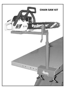
**Chain Saw Kit** - Lay the chain saw on the support pad with the blade positioned between the clamp supports. The support pad can be adjusted to accommodate different lengths of chain saws. Use the clamp lever to secure the chain saw blade. Adjust the screw behind the blade to get enough pressure to hold the blade. Secure the chain saw base to the support pad with tie downs using the holes in the support pad.
