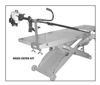
**Weed Eater Kit** - Attach the weed eater in the holder as shown and tighten the knob. It is best if the weed eater is attached somewhere near its balance point. The holder can be pivoted up and down by loosening the 3/8-16 socket head cap screw and the #8-32 socket head set screw with cup point. The holder can be rotated by loosening the knob.
