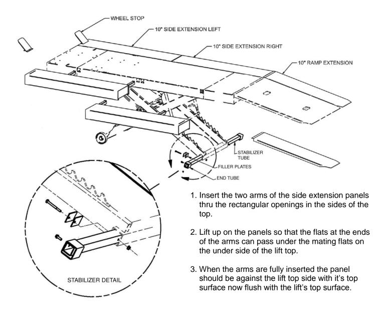
4. Wheel stops and ramp extensions are mounted as shown using the slots found at the ends of the extensions panels.
