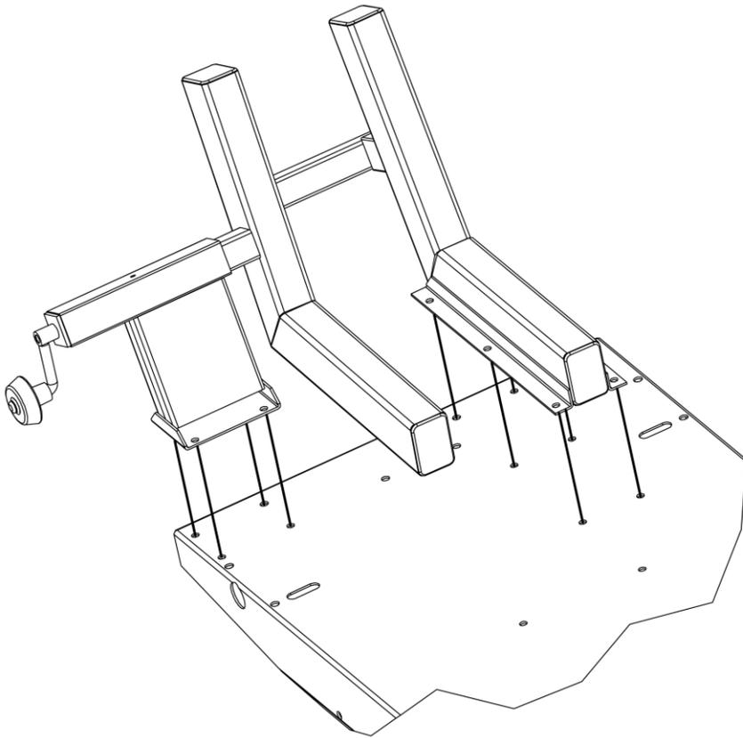
The CV-17 Cycle Vise mounts directly onto most Handy Lifts bought after January 1, 1994. Some lifts have more than one vise mounting location, allowing you to better position your bike on the lift depending on the type of service you are doing. The Cycle Vise has a removable wheel stop, this allows the user to remove the wheel stop and then be able to remove the front wheel of the motorcycle if necessary.
