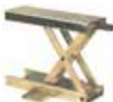
MC450 Center Lift Jack Use on lift or on floor 5-1/2" W x 16" L, 1100 lb. cap. Min Ht. 3-1/2", Max Ht. 13"
