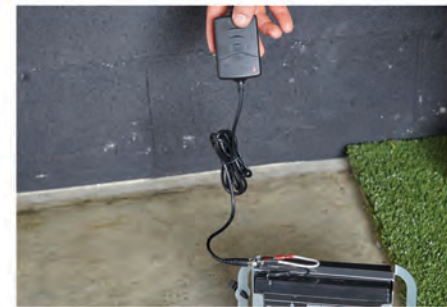
CHARGING REMOVED BATTERY
