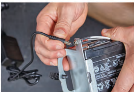
CHARGING REMOVED BATTERY
