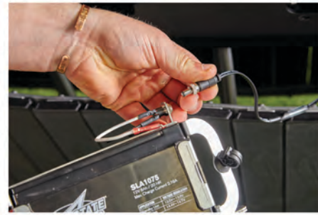
CHARGING REMOVED BATTERY
