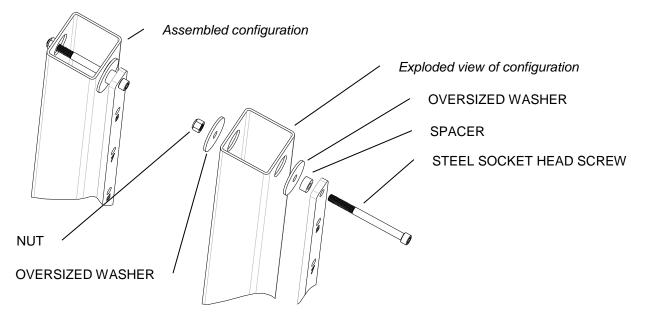
1-2 If not using existing rack holes, drilling is necessary. Please follow these instructions: measure a distance of 37 in. and drill clearance holes for 3/8" fasteners into existing rack. *Fasten the bottom first* of the sliding rail as shown below using 5/16" hex key using the fasteners included. Slide pulley assembly through top of rail and then fasten the top of sliding rail as shown below.
