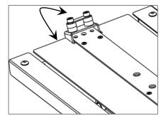
b) Seat Installation: Tilt the Seat slightly upward to allow the front Rollers to engage the channel. Then, lift the rear level and, while engaging the Seat Lock Release Lever, slide the seat onto the Baseplate as shown.
