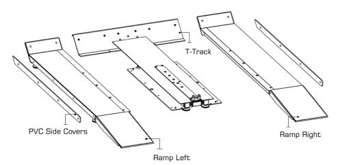
a) Bolt the T-Track to the Main Frame as shown, using 3x M10x20mm Bolts[20], 2x M10 Nylock Nut[25] and 3x M10 Washers[28]. Secure tightly.
