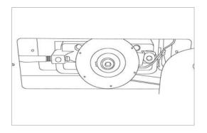
Using a long tool, push out the rear end cap as pictured below left. This will give you access to the tank
