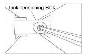
Note: Do not over tighten tank Bolts.
