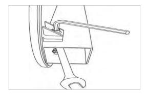
Using a 6mm Allen Key, tighten the Belt using the Tank Tensioning Bolt until the belt no longer slips during hard rowing.
