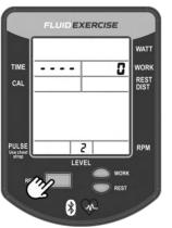
Turn handle to Level 2. Press Reset. Display will now show Level 3. Level 2 Calibration is complete.
