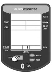
Turn handle to Level 1. Press Reset. Display will now show Level 2. Level 1 Calibration is complete.
