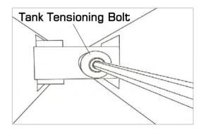
Note: Do not over tighten Tank Bolts.
