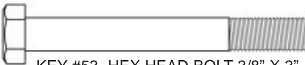
KEY #53 HEX HEAD BOLT 3/8" X 3" PARTIAL THREAD QTY. 7
