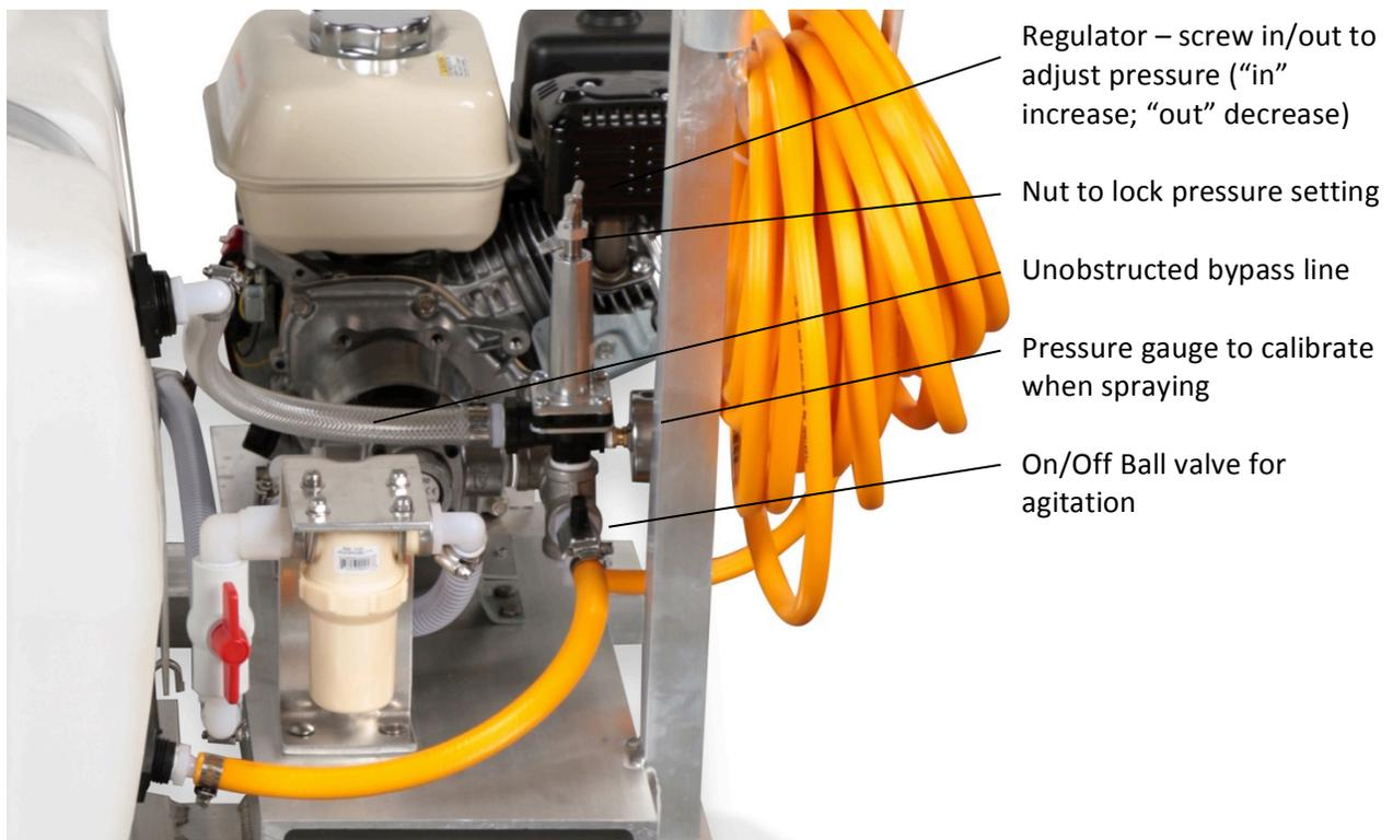
Regulator – screw in/out to adjust pressure (“in” increase; “out” decrease)
