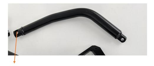
Use 5/16-18 allen bolts to attach both bars to bumper body do not tighten completely
