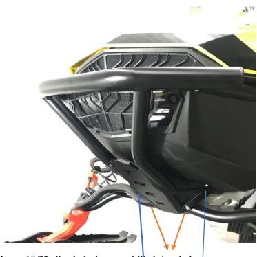
Insert 10/32 allen bolts into pre drilled rivet holes
