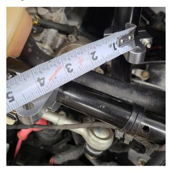
**Step 8:** Install the clamp onto the steering stabilizer. Position the clamp like pictured, measure 3" from the end of the stabilizer to the bracket. Tighten the bolts on the bracket.
