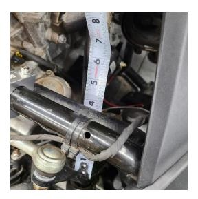
**Step 6:** Install the bracket onto the steering shaft, use blue Loctite on the bolts.
