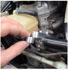
**Step 5:** Measure from the bottom of the steering shaft and make a mark at 5.5" on the round steering shaft.
