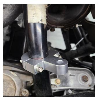
**Step 7:** Turn the handlebars all the way to the right (sitting on the bike). Measure 4.75" Center to center of both aluminum brackets. Tighten the bolts on the bracket.
